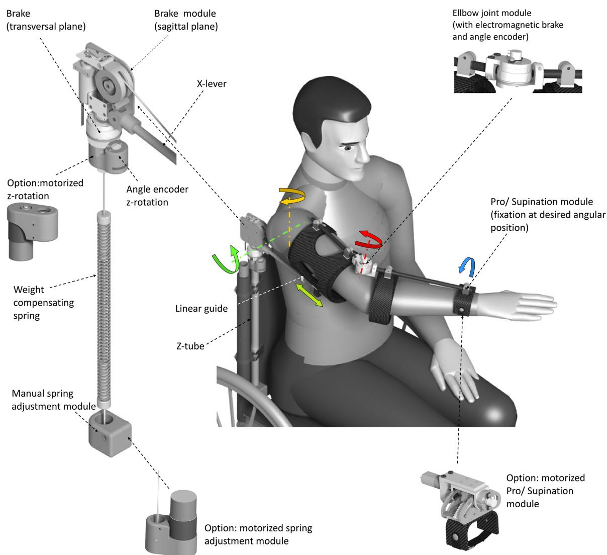
Figure 1: Digital mock-up of the orthosis worn by a manikin and mounted on a wheel chair. The colored arrows depict the mechanical DoF. The main mechanical components and optional modules are illustrated by detailed 3-D graphics.
