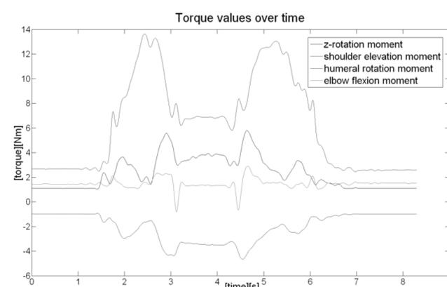
Figure 3: Torque values on each DoF after a dynamic analysis of the "Drinking" task. The additional force of a bottle was considered with 5N (500ml).
