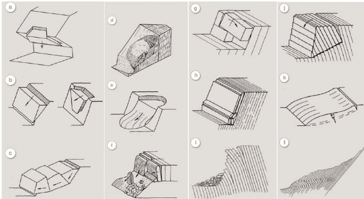
Figure 1: Rock slope failure mechanisms (from: Poisel & Preh, 2004)
