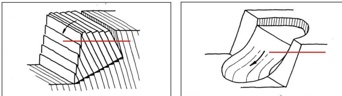
Figure 1: Extensometer for monitoring toppling and rotational failure
