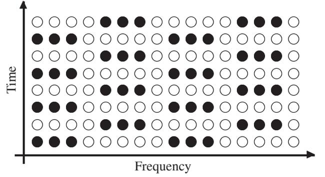
Fig. 2. An illustration of the proposed pilot arrangement with  $K = 16$ ,  $L = 2$ , and  $D = 2$  ('o' represents data symbols and '•' represents pilot symbols). Only the central pilot in each block is non-zero. The offset  $k_0$  is chosen equal to 0 and 4 in the even and odd symbol periods, respectively.
