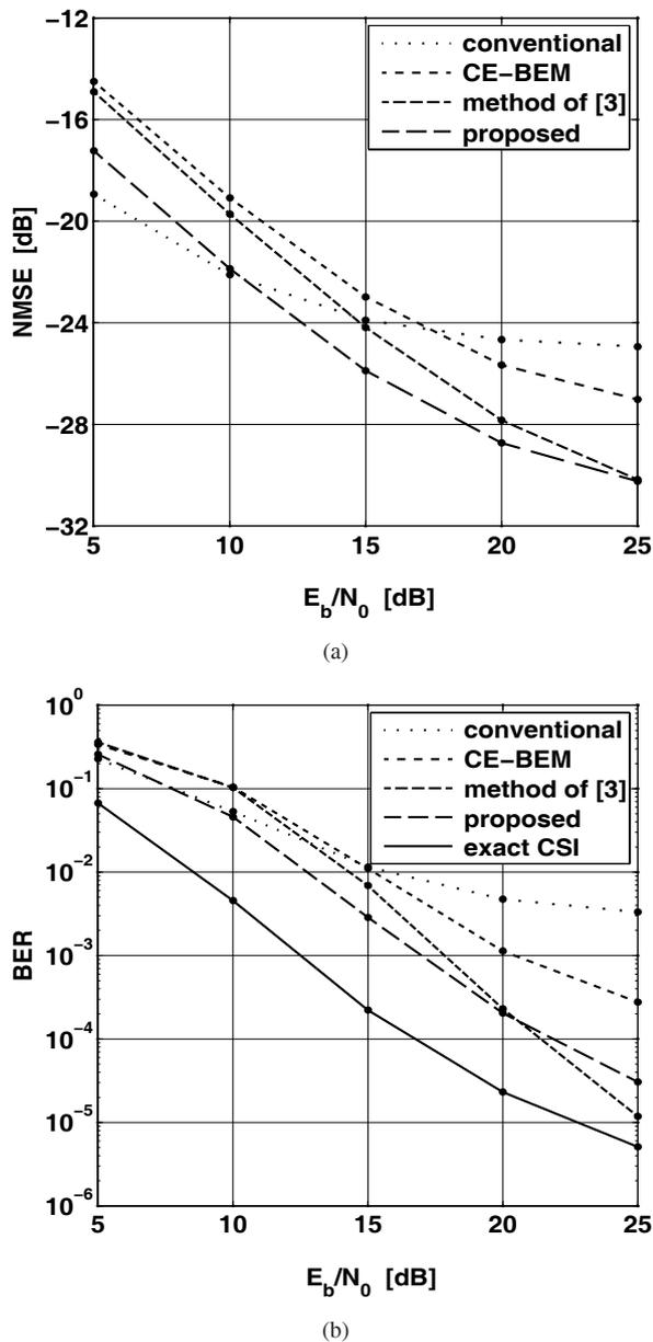
Fig. 4. (a) NMSE versus SNR and (b) BER versus SNR for a fixed receiver velocity of 300 km/h.
