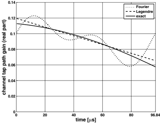
Fig. 1. A typical channel tap (real part) across one OFDM symbol, the normalized Doppler equals 0.2.
