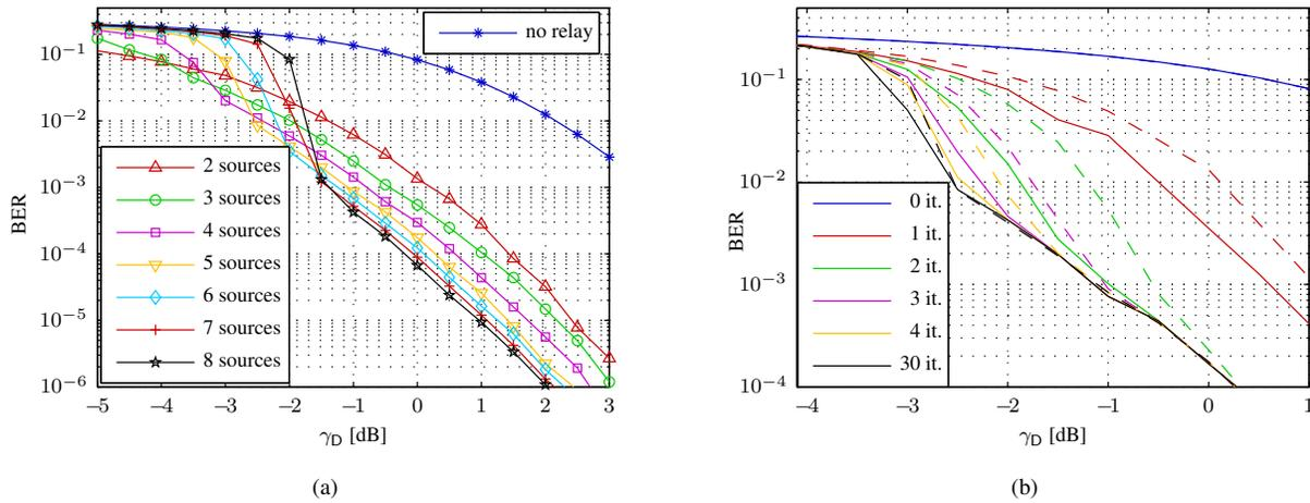
Fig. 4. Symmetric Gaussian MARC: (a) BER performance and (b) decoder convergence with serial (solid) and flooding (dashed) schedules.
