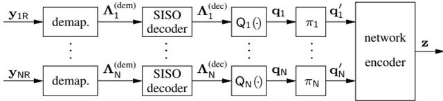
Fig. 2. Relay block diagram.
