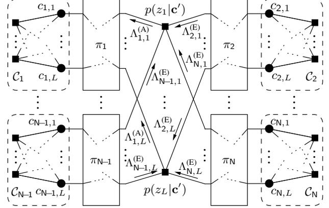
Fig. 3. Factor graph of the overall code.
