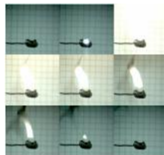
Fig. 4: Heat transfer onto a single plastic resin particle from a high energy laser shot (30 J). Recording times of photos (from top to bottom): 0ms, 1ms, 38ms, 41ms, 44ms, 50ms, 62ms, 77ms, 89ms.
