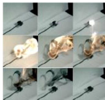
Fig. 3: Heat transfer onto a single plastic resin particle from a low energy laser shot (5 J). Recording times of photos (from top to bottom): 0ms, 1ms, 2ms, 24ms, 33ms, 39ms, 48ms, 66ms, 447ms.
