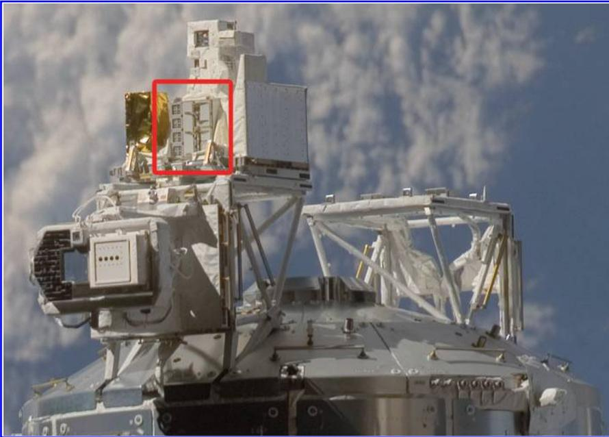
**FIG. 1.** EXPOSE-E experiment carrier (framed) attached to the EuTEF external platform of the European Columbus laboratory. Color images available online at [www.liebertonline.com/ast](http://www.liebertonline.com/ast)
