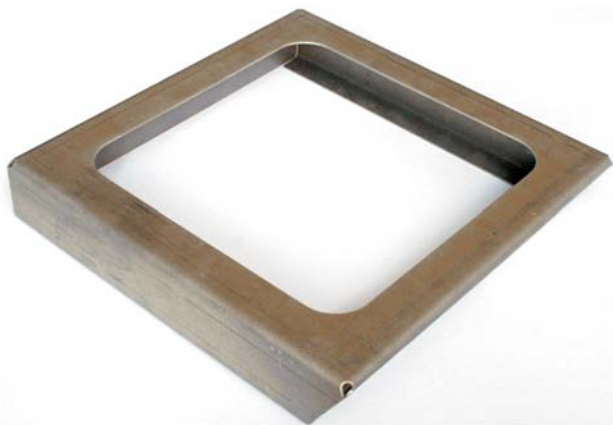
Figure 7 Bending part made of AZ31 with 6 bends with ~250 mm length
