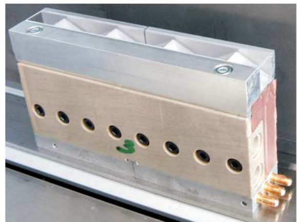
Figure 2 Diode laser inset with 100 mm length
