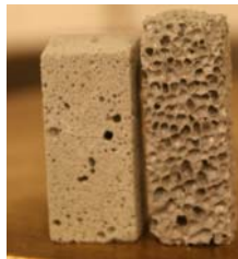
Figure 8. Two different types of foam glass aggregate prisms left fine pores, right coarse pores.
