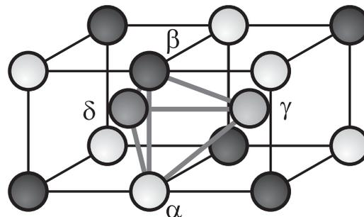
**Figure 1** The irregular tetrahedron (IT) cluster in the BCC lattice.
