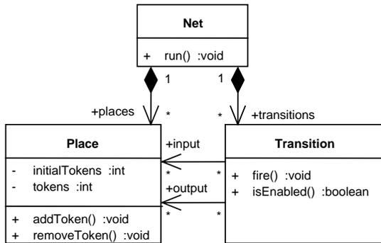
Figure 2. Metamodel of Petri Net DSML
