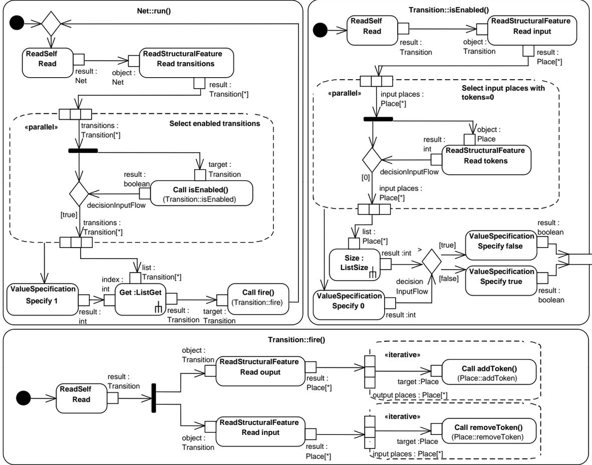
Figure 3. Semantics specification of Petri Net DSML using fUML
