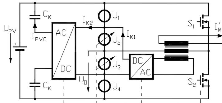
**Fig. 3.** Innovative solar inverter array with active input ripple compensation and dynamic power storage in divided DC-link capacitors
