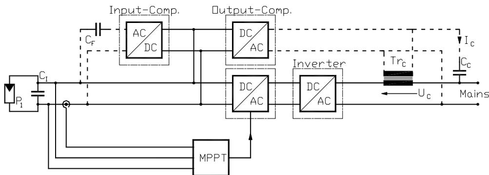
**Fig. 1.** Innovative solar inverter array with active ripple compensation and filtered power-line interface (series or parallel line interfacing by  $Tr_c$  or  $C_c$ , optionally)
