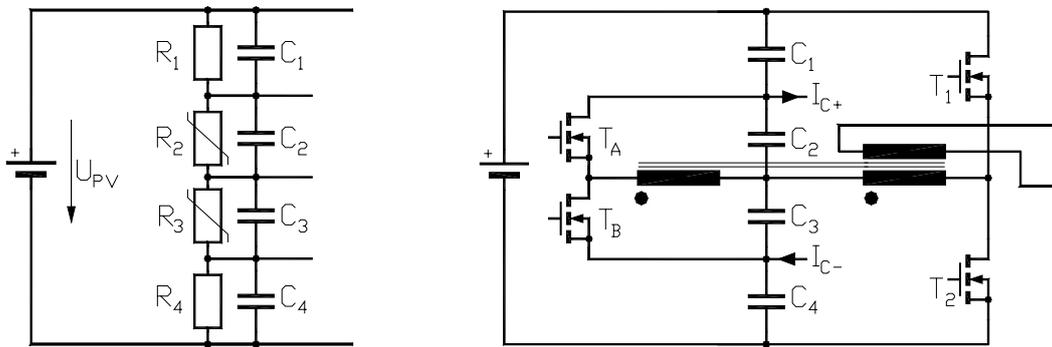
**Fig. 8.** Balancing solutions: a: resistive and b: transformer coupled with active control
