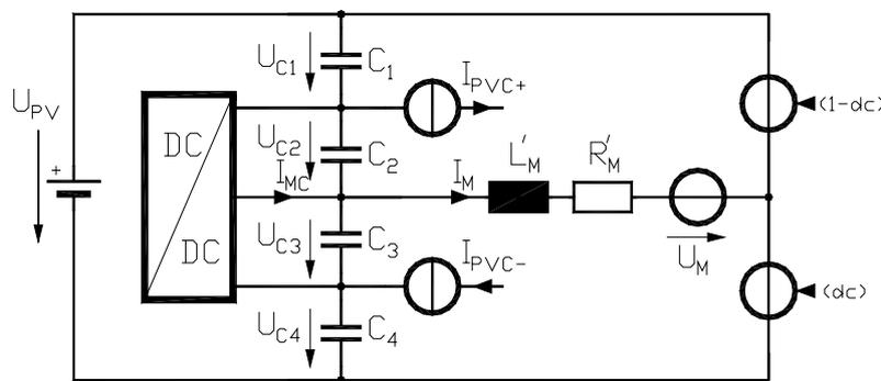
**Fig. 5.** Active energy recuperation of the compensator power in case of mains compensation
