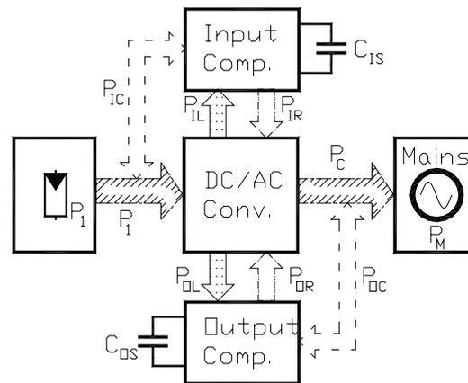
**Fig. 2.** Energy flow in a full compensated solar inverter arrangement
