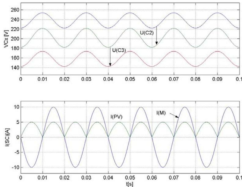
**Fig. 6.** System behavior in solar array side without compensator and input filter capacitor usage: The upper picture shows the capacitive voltage divider, while the input current shape  $I_{PV}$  and the load current  $I_M$  are shown below (green line:  $U_0$ )
