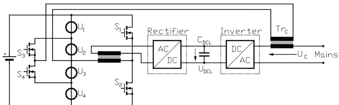
**Fig. 4.** Innovative solar inverter array with active mains current ripple compensation
