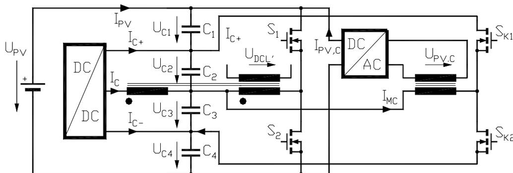
**Fig. 7.** Input current ripple compensation, dynamic current sharing
