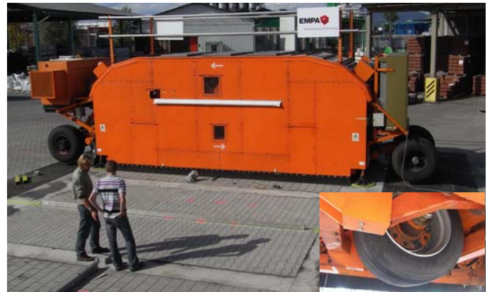
Figure 5. New Mobile Load Simulator MLS10 with super single tires.
