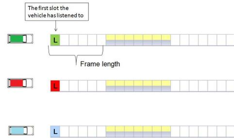
Fig. 4. Several vehicles turned on during one frame duration might attempt to gain the same NTS due to the same perception of the frame (unintended slot reuse)
