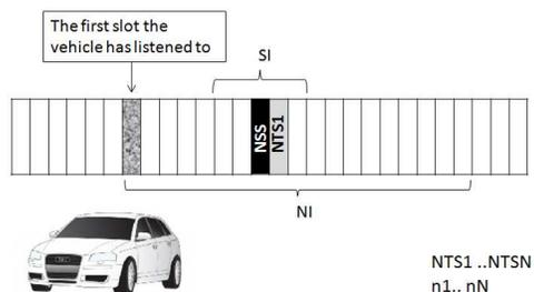
Fig. 1. STDMA slot assignment for network entry phase.
