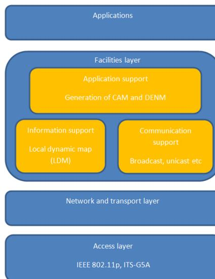
Fig. 3. Facilities Layer Architecture
