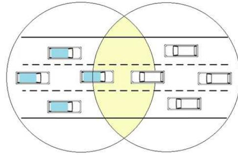
Fig. 5. As soon as the two clusters begin to merge it might happen that vehicles from Cluster A have the same NTS as other cars from Cluster B. In this scenario packet collisions will occur.
