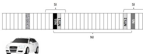
Fig. 2. STDMA slot assignment for first frame phase.
