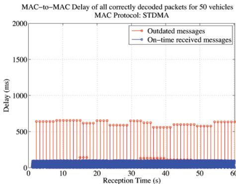
Fig. 2. STDMA MAC-to-MAC delay of all correctly decoded packets vs. reception time for lightly-loaded scenarios (50 vehicles)
