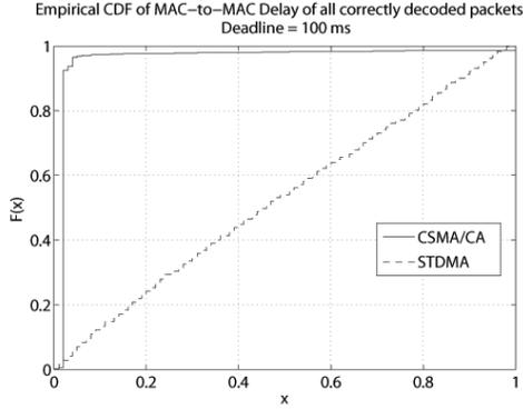
Fig. 6. Empirical CDF of MAC-to-MAC delay of all correctly decoded packets for 100 ms deadline in heavily-loaded scenarios (400 vehicles)
