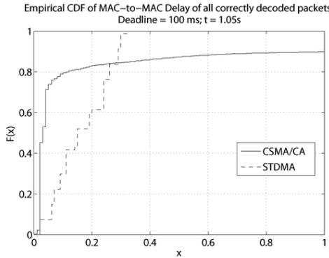
Fig. 7. Empirical CDF of MAC-to-MAC delay of all correctly decoded packets for 100 ms deadline in heavily-loaded scenarios (400 vehicles) for  $t=1.05$  s
