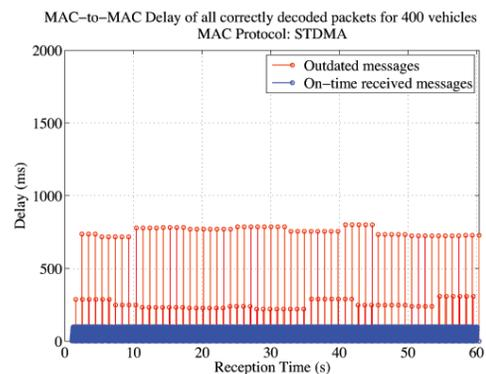
Fig. 5. STDMA MAC-to-MAC delay of each correctly decoded packet vs. reception time for heavily-loaded scenarios (400 vehicles)
