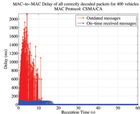
Fig. 4. CSMA/CA MAC-to-MAC delay of each correctly decoded packet vs. reception time for heavily-loaded scenarios (400 vehicles)
