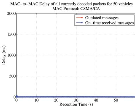
Fig. 1. CSMA/CA MAC-to-MAC delay of all correctly decoded packets vs. reception time for lightly-loaded scenarios (50 vehicles)
