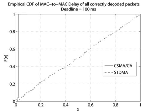
Fig. 3. Empirical CDF of MAC-to-MAC delay of all correctly decoded packets for 100 ms deadline in lightly-loaded scenarios (50 vehicles)
