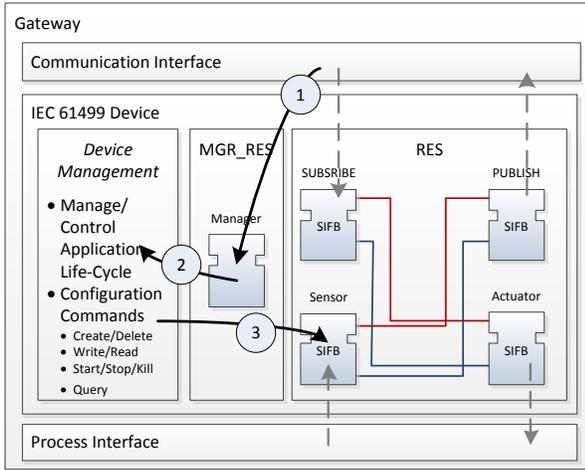
Fig. 4. IEC 61499 standard-compliant reconfiguration approach
