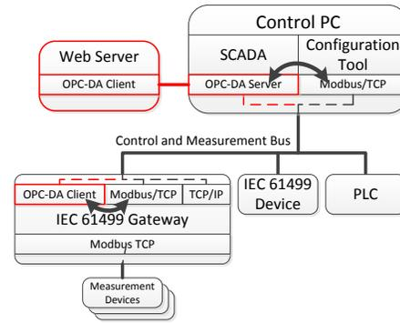
Fig. 5. Reconfiguration of SCADA communication
