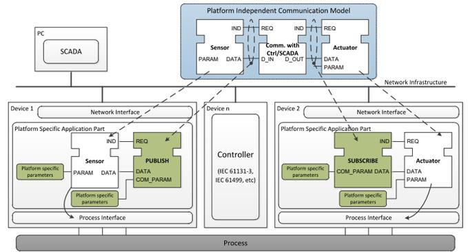
Fig. 3. MDA mapped to the IEC 61499 reference model [22], [26], [27]
