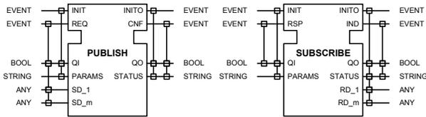
Fig. 2. Generic PUBLISH/SUBSCRIBE SIFBs for uni-directional transactions according to IEC 61499-1 Annex E [2]
