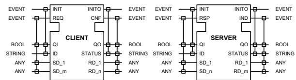
Fig. 1. Generic CLIENT/SERVER SIFBs for bi-directional transactions according to IEC 61499-1 Annex E [2]
