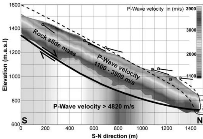
Figure 3. Seismic cross section (N-S direction), close to A-A'.
