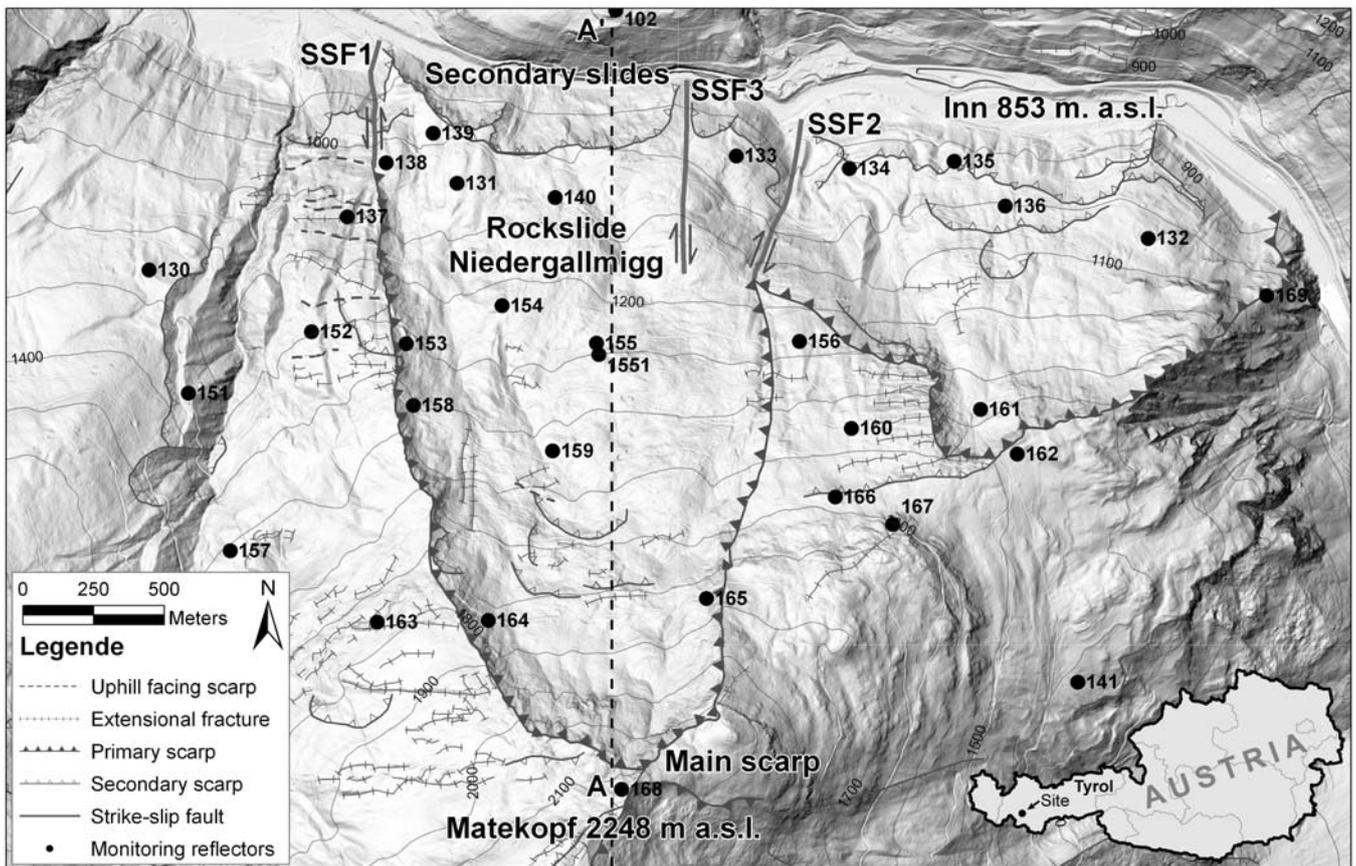
Figure 1. Hillshade map of the deep-seated rock slide system Niedergallmigg (Austria) showing primary and secondary scarps, strike-slip faults (SSF1, SSF2, SSF3), geodetic monitoring targets and the trace of the cross section A-A'.
