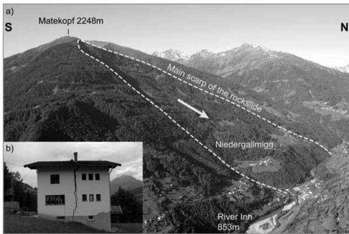
Figure 2. a) Rock slide system Niedergallmigg with the main head scarp, the river Inn and the location of the village Niedergallmigg, b) damaged house located close to the western boundary of the slide.
