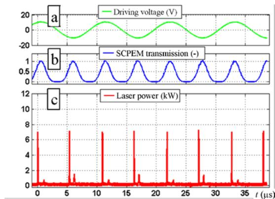
Fig. 5. Experimental results for SCPEM mono-mode-operation. Driving voltage (a), relative optical transmission (b) and laser output pulses (c). Pulse repetition frequency 183.6 kHz.
