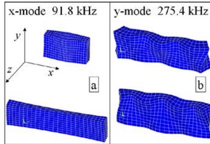
Fig. 2. Finite-element-simulation (with the program ANSYS) of two different eigenmodes of a y-excited LiTaO<sub>3</sub>-crystal with dimensions of 28.6x9.5x4 mm: x-eigenmode at 91.8 kHz (a) and y-eigenmode at 275.4 kHz (b).
