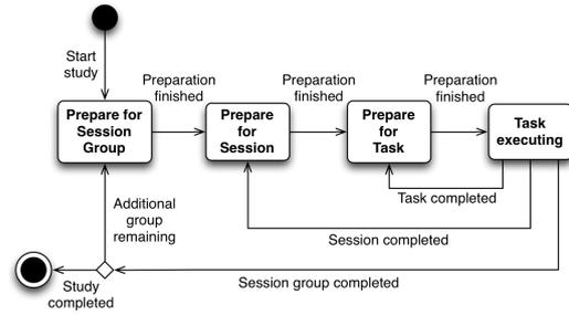
Figure 3: **Evaluation process.** Simplified state machine that is run by the EvaluationManager during an evaluation.
