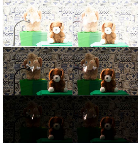
Figure 3: A sample from a multi-exposed stereo data set. First row: over-exposed left and right views (exposure = 1/3 s); Second row: normal-exposed left and right views (exposure = 1/50 s); Third row: under-exposed left and right views (exposure = 1/400 s).
