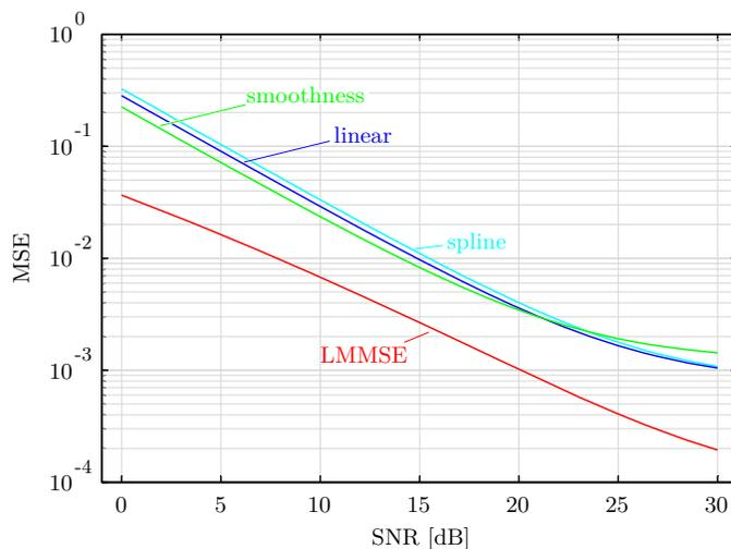
Fig. 3. Channel estimation MSE as a function of SNR at an UE speed of 100 km/h.
