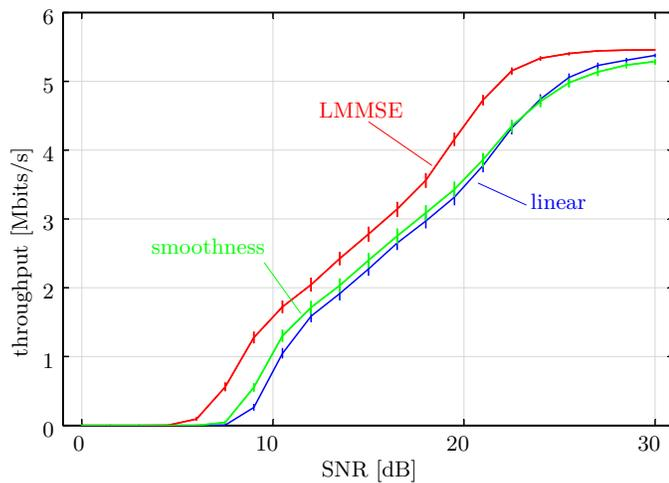
Fig. 4. Coded throughput. We transmitted 1500 subframes and calculated the 95% confidence intervals as shown above.
