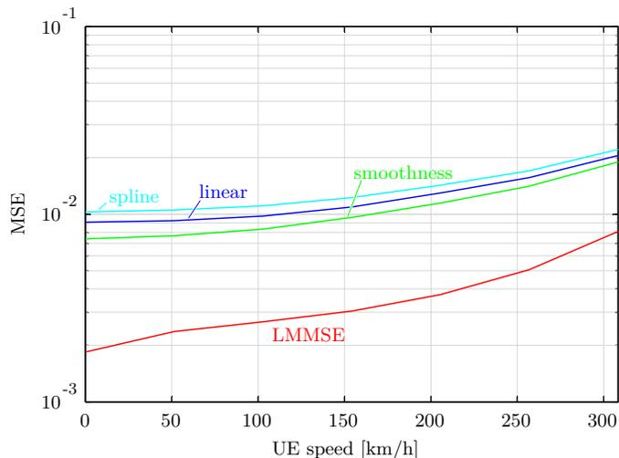
Fig. 2. Channel estimation MSE as a function of UE speed with SNR = 15 dB.
