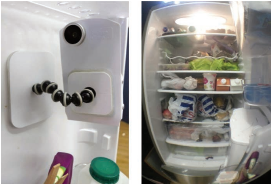
Fig. 1. FridgeCam system attached to the door (left) and picture of the inside of the fridge taken by the camera (right).
