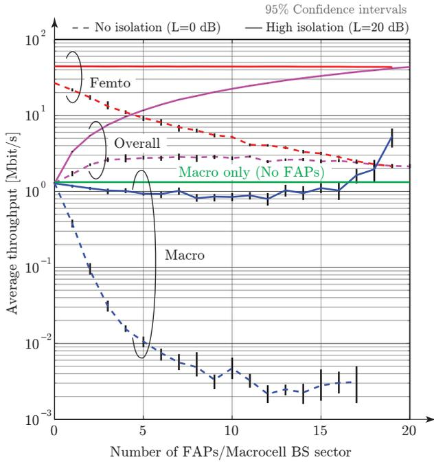
Fig. 4: Average user throughput versus FAP density. 'Macro' refers to macrocell-attached users in a femtocell-enhanced network. 'Macro only' is the reference case without FAP employment.
