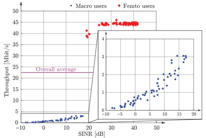
Fig. 5: Individual throughput values: Blue dots in the lower left corner correspond to macrocell-attached users, red dots in the upper right corner denote the femtocell users.
