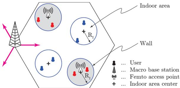
Fig. 1: User distribution in macrocell sector. Users are spread uniformly within homogeneously distributed indoor areas of radius  $R_I$ . FAPs are positioned exactly at centers of the indoor areas (denoted by '+' ) and attach only the users of the corresponding area.
