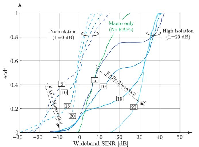
Fig. 3: Wideband-SINR distributions of various femtocell densities (the boxed numbers denote the number of femtocells per macrocell sector) for No Isolation- and High Isolation scenario (dashed and solid lines, respectively). The reference case is denoted as "Macro Only".
