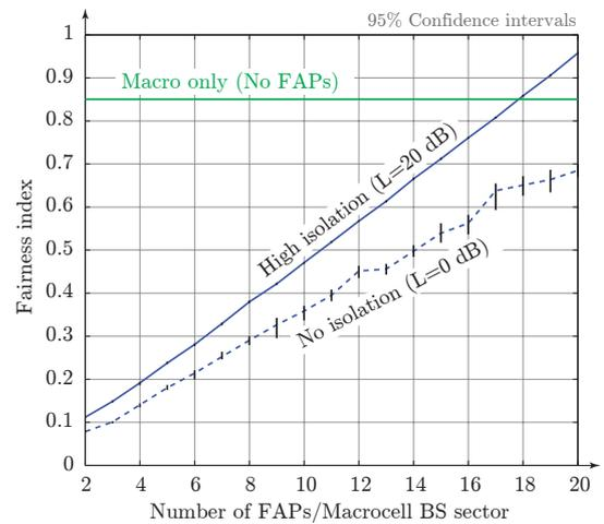
Fig. 6: Jain's Fairness Index plotted versus the femtocell density for HI- and NI scenario (solid and dashed line respectively).
