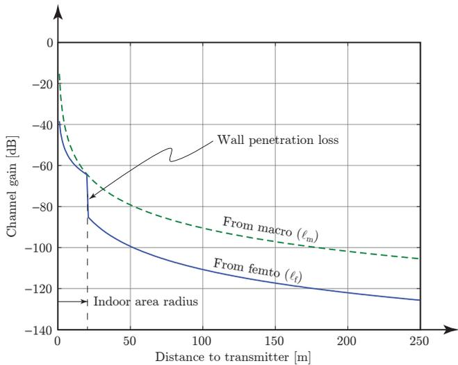
Fig. 2: Channel power gain of model according to [15] (dashed line) and dual slope propagation model (solid line). Simulation parameters are listed in Table I.
