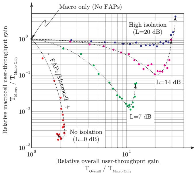
Fig. 7: Macrocell- and overall average user throughput gain related to the 'Macro Only' scenario. Dashed arrows point in the direction of increasing FAP density (ranging from 0 to 20 FAPs/Macrocell BS).
