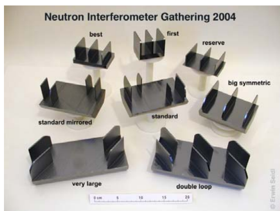
Fig. 1 All neutron interferometers used at the Vienna TRIGA reactor or at the high flux reactor of the ILL, Grenoble were manufactured and tested at the Atominstitut.
