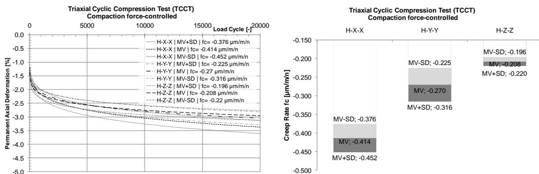
Figure 7. TCCT results for force-controlled compaction: Creep curve (left), and creep rate (right).
