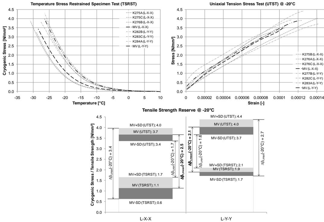
Figure 3. TSRST results (upper left), UTST results (upper right) and tensile strength reserve (below).
