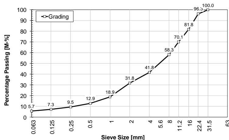
Figure 1. Grading curve.
