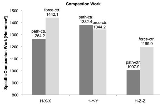
Figure 10. Compaction work of HMA-slabs used for TCCT specimens.
