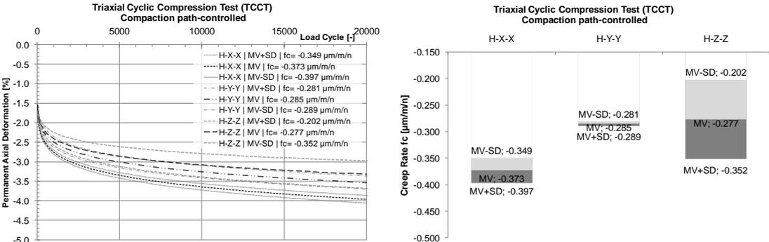
Figure 5. TCCT results for path-controlled compaction: Creep curve (left), and creep rate (right).
