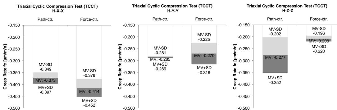
Figure 9. TCCT results – path- vs. forced-controlled compaction: creep rates.
