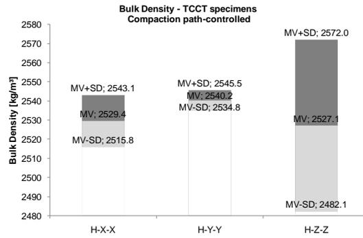
Figure 6. Bulk density of path-controlled compacted TCCT specimens.
