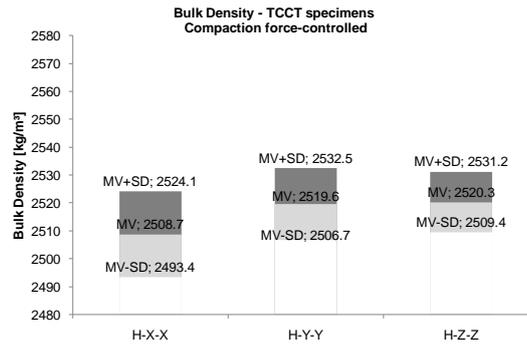
Figure 8. Bulk density of force-controlled compacted TCCT specimens.
