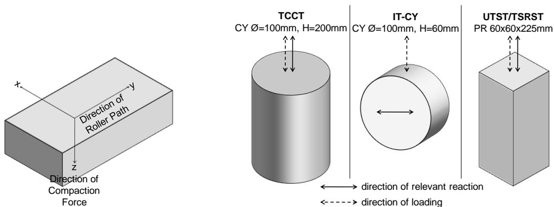
Figure 2. Coordinate system of compaction (left) and principal directions of testing (right).
