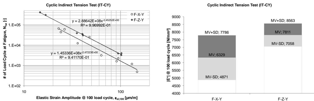
Figure 4. IT-CY results: Fatigue function (left), and stiffness (right).
