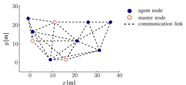
Fig. 1. Example of a sensor network with ANs and MNs.
