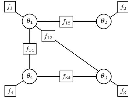
Fig. 3. Example factor graph of a network with node set  $\mathcal{I} = \{1, 2, 3, 4\}$ . Variable nodes and factor nodes are depicted by circles and rectangles, respectively. The shorthands  $f_i \triangleq f(\boldsymbol{\theta}_i)$  and  $f_{ij} \triangleq f(\mathbf{c}_{ij}|\boldsymbol{\theta}_i, \boldsymbol{\theta}_j)$  are used.
