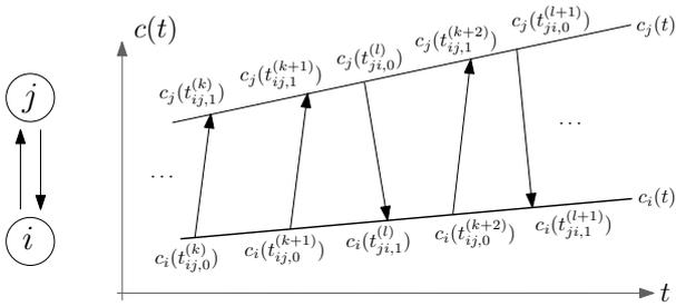
Fig. 2. Local clock functions  $c_i(t)$  and  $c_j(t)$ , local time measurements (time stamps), and corresponding packet transmissions for nodes  $i$  and  $j$ .
