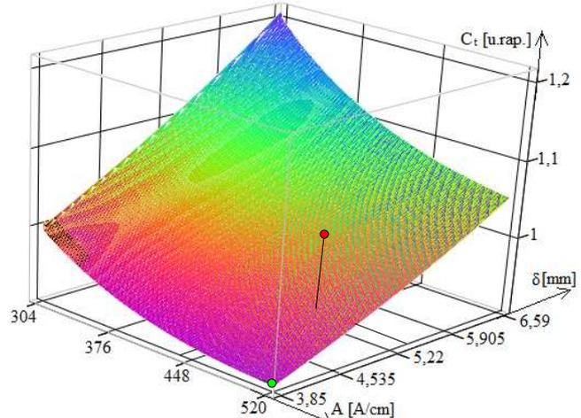
Fig. 7. Total cost variation depending on the current blanket and the air gap size for the 1000 rot/min hydrogenerator.
