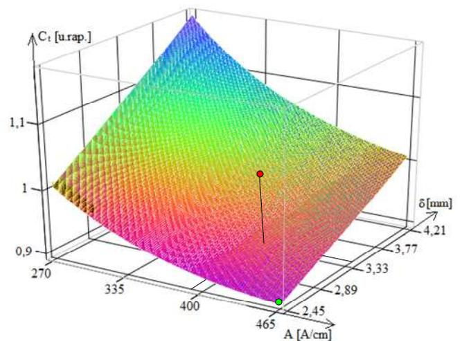
Fig. 5. Total cost variation depending on the current blanket and the air gap size for the 600 rot/min hydrogenerator.
