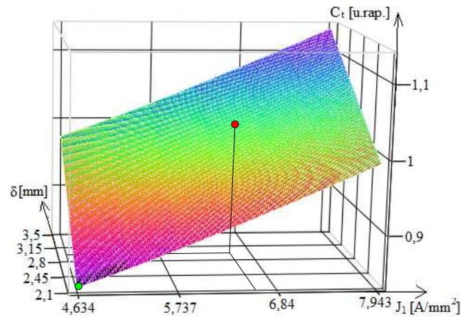
Fig. 11. Total cost variation depending on the statoric winding current density and the air gap size: the 500 rot/min hydrogenerator.
