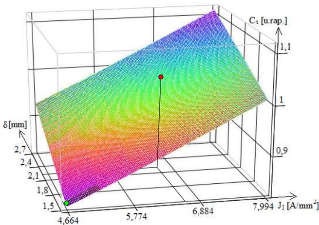
Fig. 8. Total cost variation depending on the statoric winding current density and the air gap size for the 250 rot/min hydrogenerator.
