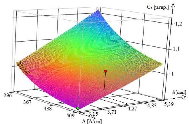
Fig. 6. Total cost variation depending on the current blanket and the air gap size for the 750 rot/min hydrogenerator.
