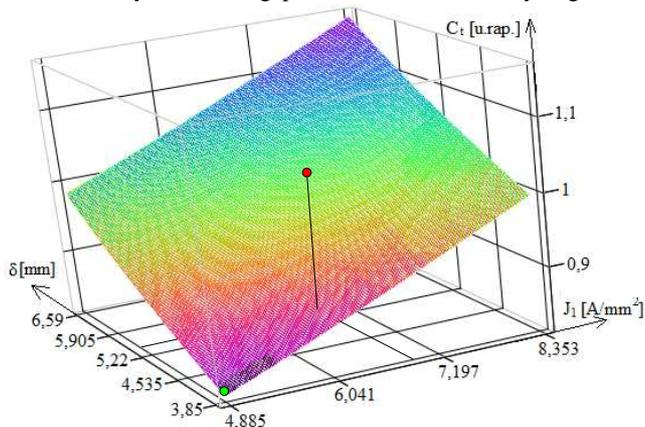
Fig. 14. Total cost variation depending on the statoric winding current density and the air gap size: the 1000 rot/min hydrogenerator
