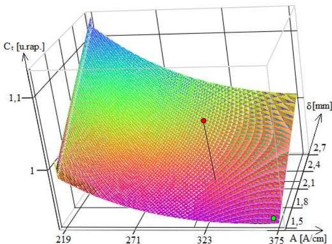
Fig. 1. Total cost variation depending on the current blanket and the air gap size for the 250 rot/min hydrogenerator.
