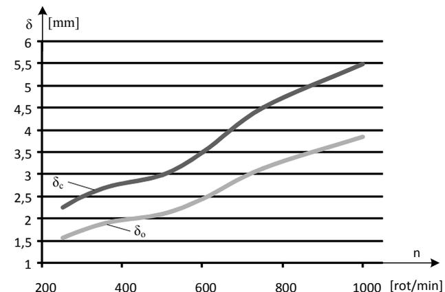
Fig. 15. Air gap size variations depending on the generator's rotation
