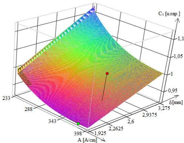
Fig. 3. Total cost variation depending on the current blanket and the air gap size for the 375 rot/min hydrogenerator.
