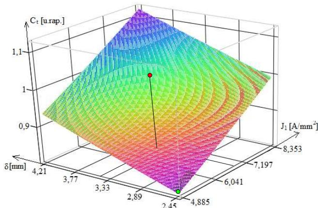
Fig. 12. Total cost variation depending on the statoric winding current density and the air gap size: the 600 rot/min hydrogenerator.
