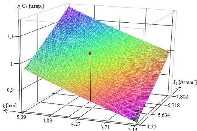
Fig. 13. Total cost variation depending on the statoric winding current density and the air gap size: the 750 rot/min hydrogenerator.
