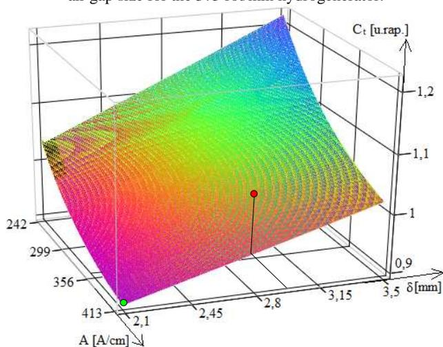
Fig. 4. Total cost variation depending on the current blanket and the air gap size for the 500 rot/min hydrogenerator.
