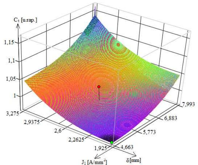
Fig. 10. Total cost variation depending on the statoric winding current density and the air gap size: the 375 rot/min hydrogenerator.
