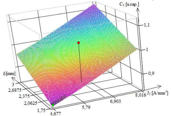
Fig. 9. Total cost variation depending on the statoric winding current density and the air gap size for the 300 rot/min hydrogenerator.
