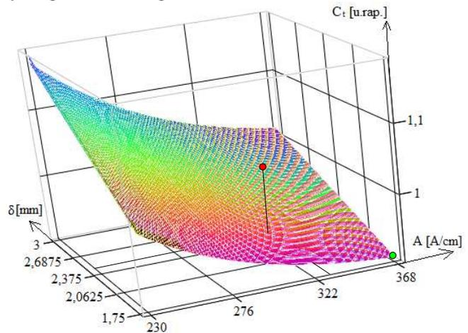
Fig. 2. Total cost variation depending on the current blanket and the air gap size for the 300 rot/min hydrogenerator.
