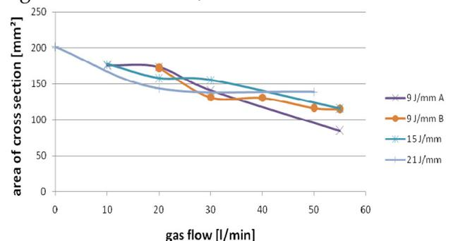
Figure 5: Area of cross section in dependency of gas flow rate
