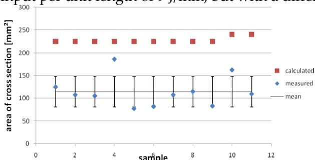
Figure 4: Comparison between measured and calculated area of cross section for a gas flow of 50 l/min, line energy 9 J/mm
