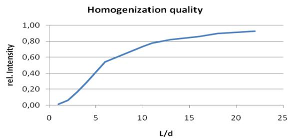
Figure 2: Relative intensity between the edge and the center of a beam at the output plane of a kaleidoscope with L length and d opening width
