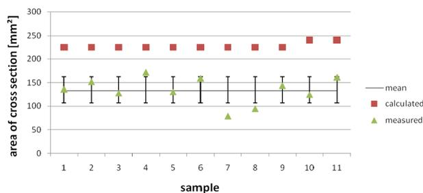
Figure 3: Comparison between measured and calculated area of cross section, line energy 9 J/mm, 30 l/min gas flow
