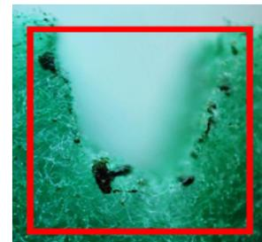
Figure 7: Evaporated area with measured rectangular, homogenized laser beam
