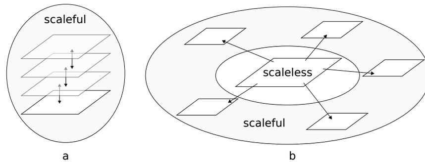
**Fig. 2.** Two types of scaleable database architecture: (a) Typical hierarchical MRDB structure (b) centralised structure with scaleless main database
