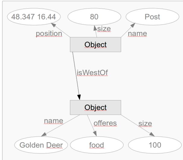
**Fig. 3.** Possible layout of a simple scaleless data structure
