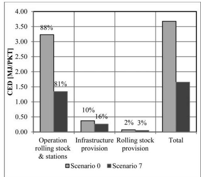
**Figure 2b.** Baseline (scenario 0) and applying all reduction measures (scenario 7) results for the CED.
