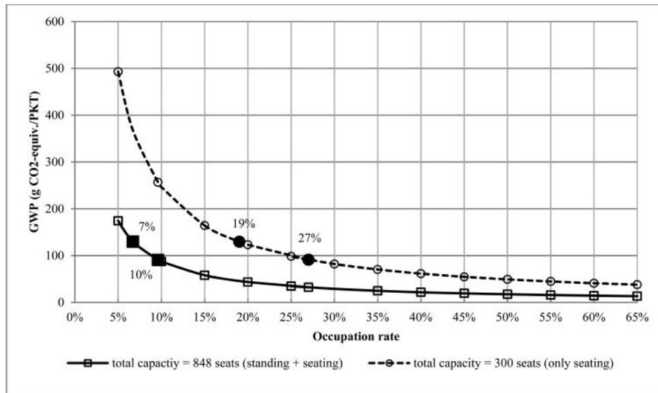
Figure 4. Influence of train occupation rate on the GHG emissions for the combined measures calculation.
