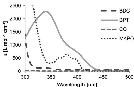
**Figure 1.** UV–vis-absorption spectra of the photoinitiators/photoinitiators **BDC**, **BPT**, **MAPO**, and **CQ** ( $1 \times 10^{-3}$  mol L $^{-1}$  for **BDC**, **BPT**, and **MAPO** and  $1 \times 10^{-2}$  mol L $^{-1}$  for **CQ** in CH $_2$ Cl $_2$ ).
