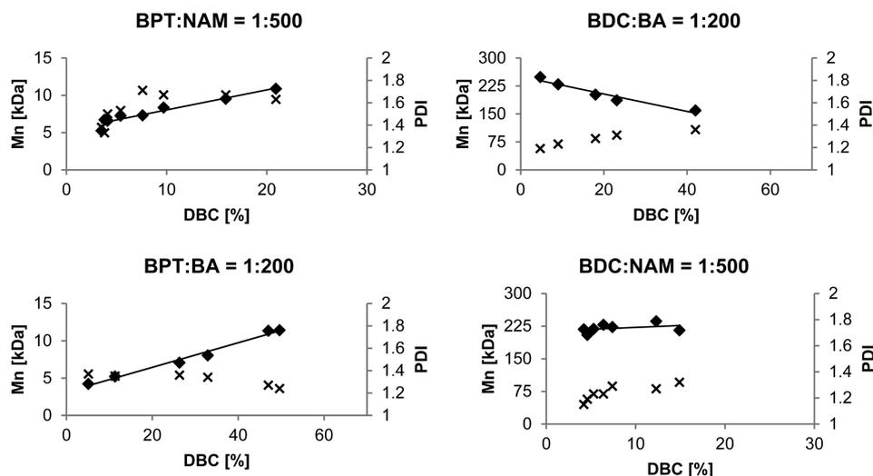
**Figure 2.** Number-average molecular weight  $M_n$  (diamonds) and PDI (crosses) versus double-bond conversion (DBC) plots for BDC and BPT with BA and NAM in bulk determined with photoreactor experiments.
