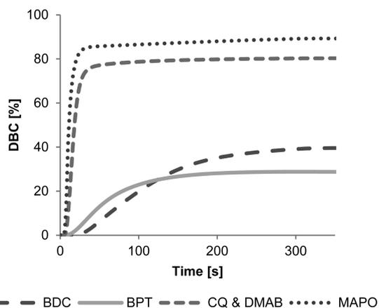
**Figure 3.** Double-bond conversion DBC [%] versus time [s] for the CRP reagents BDC and BPT and for the photoinitiator systems MAPO and CQ/DMAB in NAM with a molar ratio of 1:500 each (0.3, 0.4, 0.5, and 0.5 wt %, respectively).
