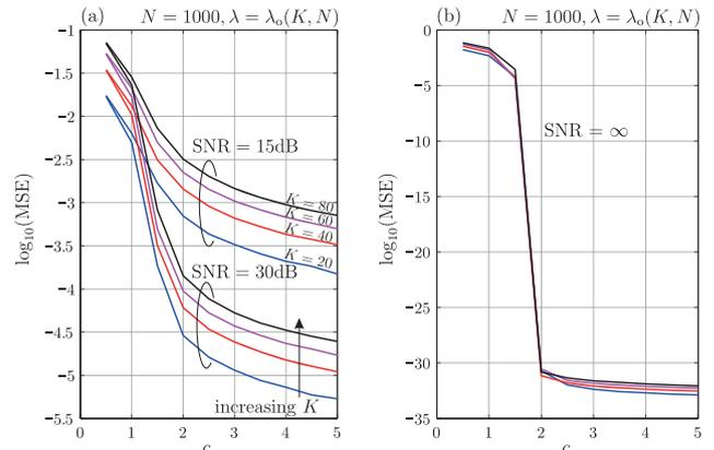
Fig. 4. (a) visualizes the MSE vs.  $c$  for various values of  $K$  and SNR. Remember that  $c$  determines the number of measurements according to (2). (b) depicts the MSE vs.  $c$  in the noiseless case. Note the distinctive threshold of  $c$  where the MSE becomes numerically zero.
