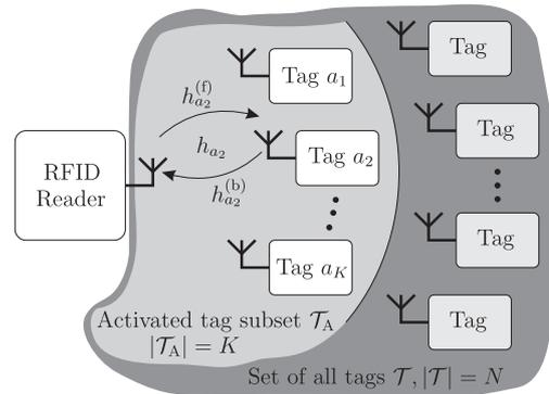
Fig. 1. Illustration of the problem scenario:  $\mathcal{T}_A$  denotes the set of activated tags that are to be identified by the reader.
