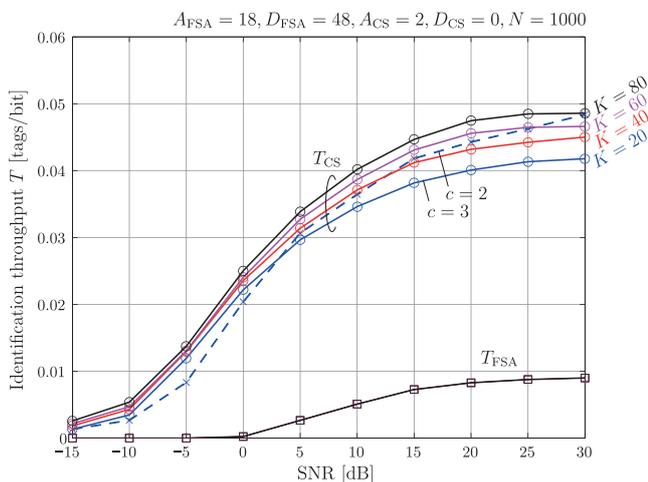
Fig. 8. Comparison of identification throughput vs. SNR.
