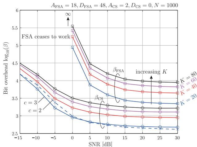
Fig. 7. Comparison of bit overhead vs. SNR.
