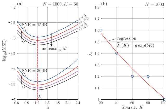
Fig. 3. (a) shows the MSE vs.  $\lambda$ . Note the convexity and the unique minimum at  $\lambda_0$ . (b) depicts the optimal value  $\lambda_0$  versus increasing  $K$ .
