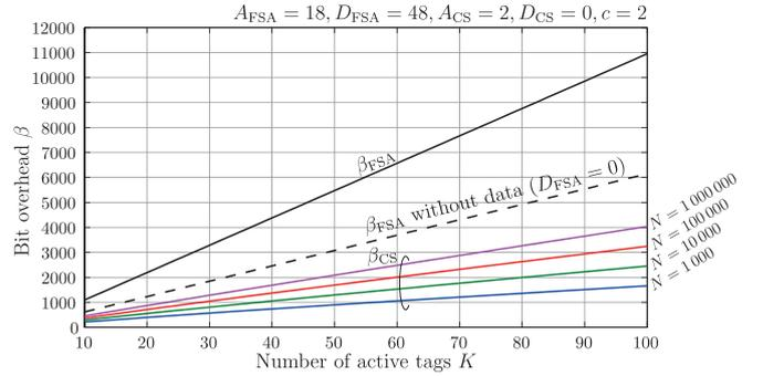
Fig. 6. Theoretically optimal (lowest possible) bit overhead for FSA (see (11)) and compressed sensing (see (10)) at infinite SNR.
