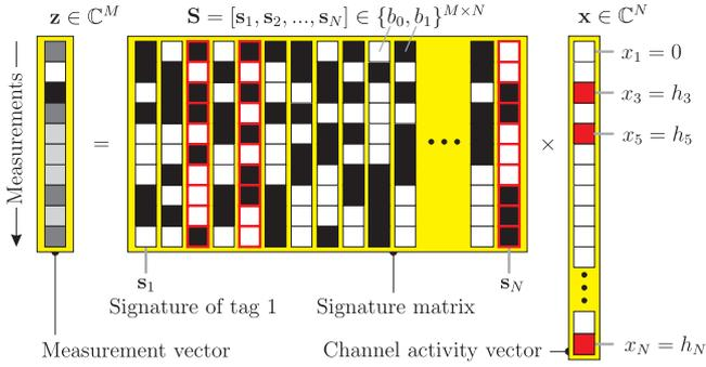
Fig. 2. Measurement process according to (5), noise omitted. Activated tag signatures selected by the non-zero elements in  $\mathbf{x}$  are highlighted.
