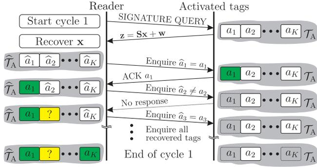
Fig. 5. Illustration of one identification cycle. Tag  $a_2$  was missed and has to be detected in a successive cycle.
