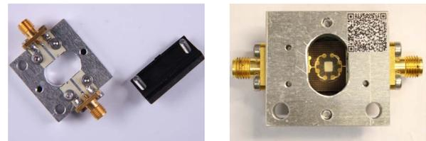
(a) Disassembled fixture. (b) Fixture's downside.
