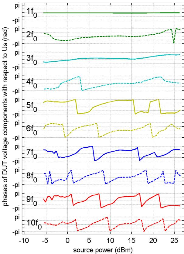
Fig. 8: Phases of DUT voltage components on the harmonic frequencies with respect to  $U_s$ .
