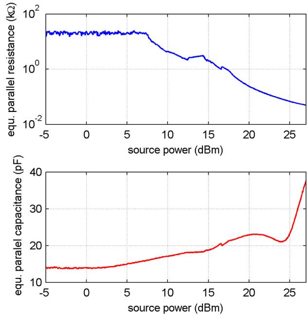
Fig. 6: Resistance and capacitance of the equivalent  $R_p$  and  $C_p$  calculated from  $S_{21}$ .
