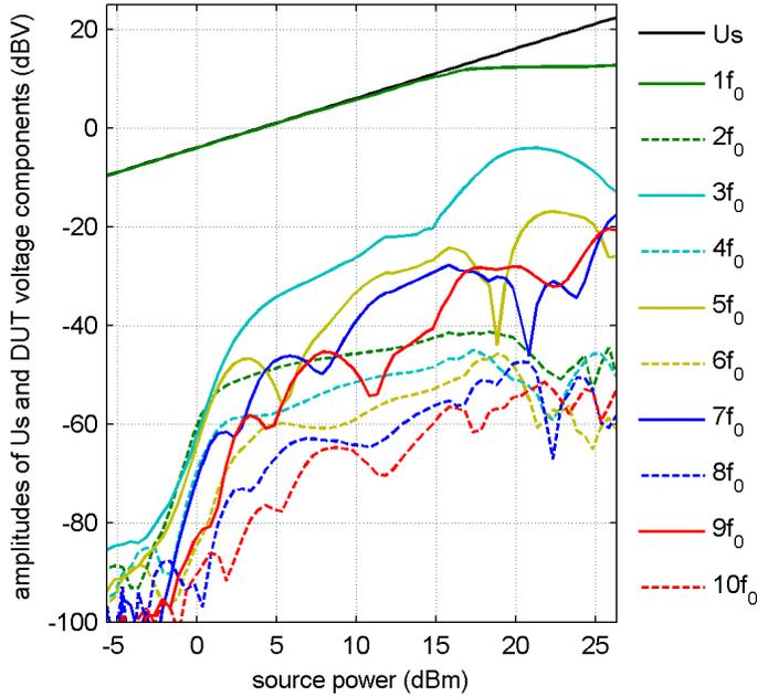
Fig. 7: Amplitude of  $U_s$  and DUT voltage components on the harmonic frequencies.
