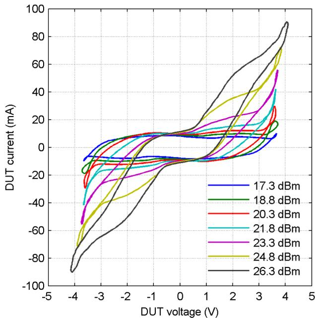
Fig. 10: Lissajous curves for high input power levels.
