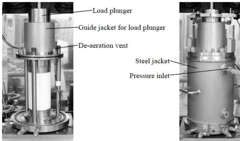
Figure 9. Main elements of a triaxial cell used for permanent deformation tests (Blab & Eberhardsteiner 2009)
