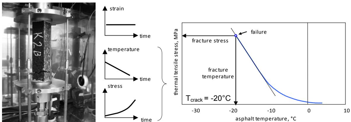
Figure 1. TSRST: experimental setup and illustration of result (Blab & Eberhardsteiner 2009)
