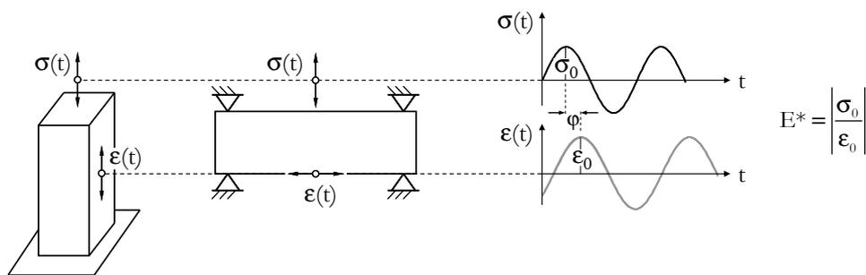
Figure 3. Stiffness modulus ( $E^*$ ) and phase angle ( $\varphi$ ) (Blab & Eberhardsteiner 2009)
