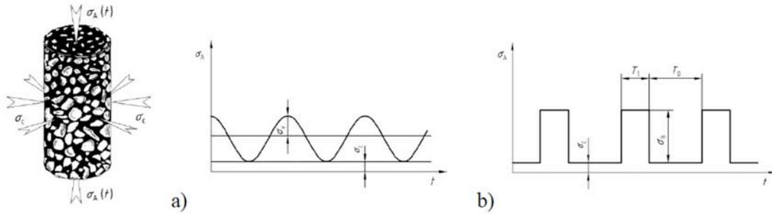
Figure 8. a) sinusoidal shaped axial loading and b) block-impulses as axial loading, both with constant confining pressure (EN 12697-25, 2008)
