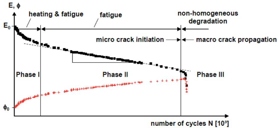
Figure 6. Phases of AC 22 fatigue curve from a strain controlled 4PBBT (acc. to: Di Benedetto et al. 2001).
