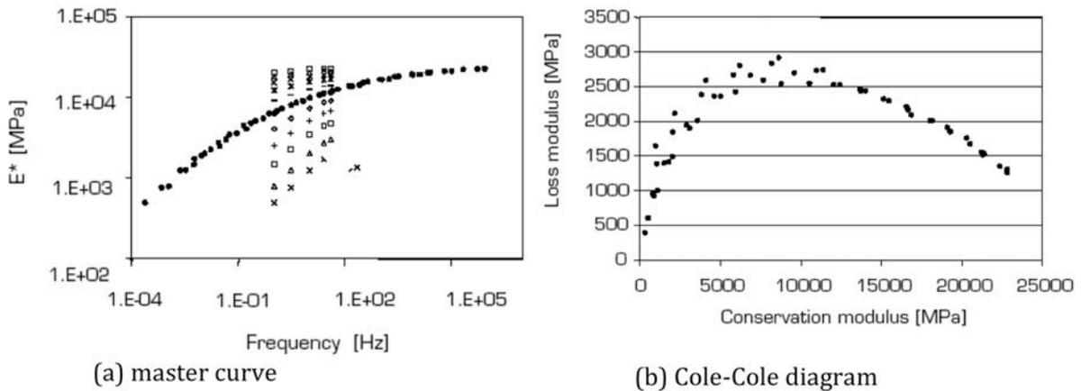
Figure 5. Stiffness master curve of SMA 11 derived from a 4PBBT
