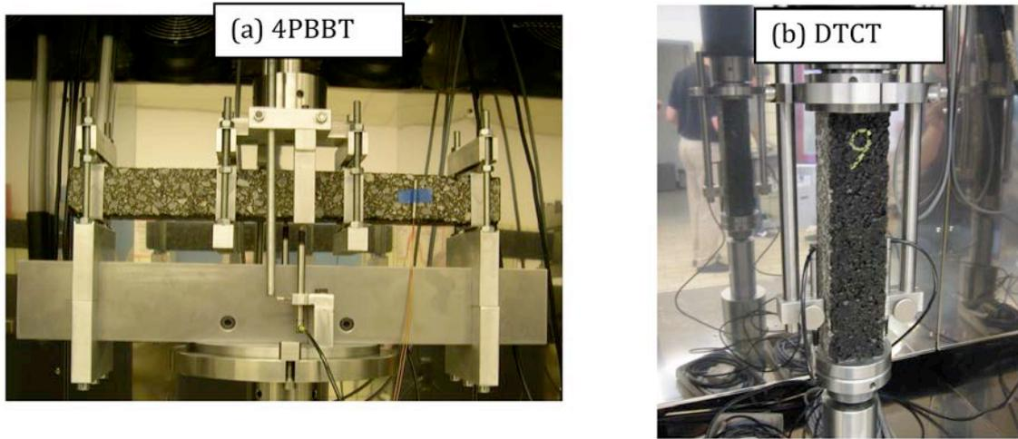
Figure 4. 4PBBT & DTCT equipment used for stiffness and fatigue testing (Blab & Eberhardsteiner 2009)
