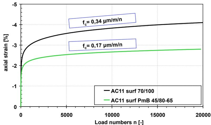
Figure 13. Creep curves for HMA type AC 11 surface with two different of binders
