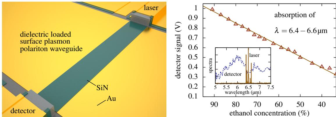
Fig. 1. Sketch of the fabricated device (left). Experiment measuring the absorption of a testing fluid (ethanol/water) with different concentrations (right). The inset shows the laser and detector spectra of the device.
