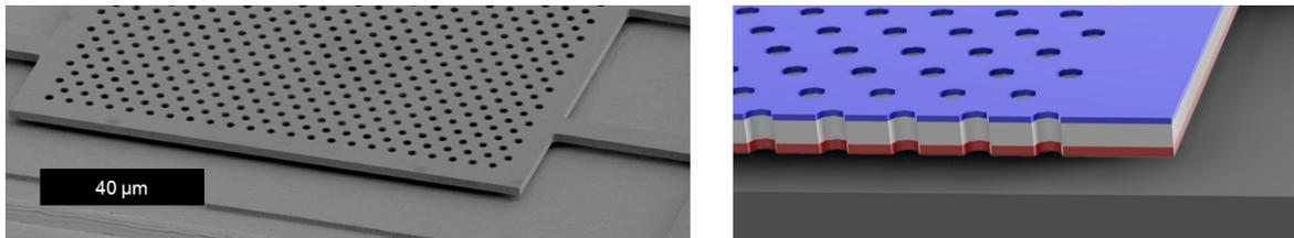
Fig. 1. Scanning electron microscopy image of a fabricated PCS-QCD and a schematic illustration of the crosssection of the PCS. Contact layers are red (bot) and blue (top), the active region is white.
