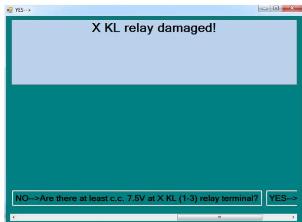
Fig. 4. Failure cause: a defect X KL relay.
