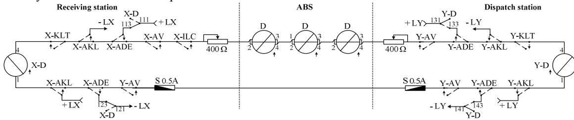
Fig. 1. Directing relays circuit.
