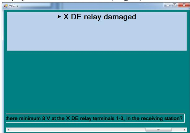
Fig. 5. Damage cause displayed by the INVBl tool: damaged X DE relay.
