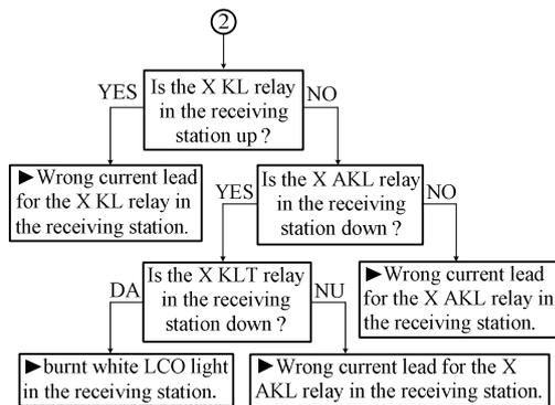
Fig. 3. Diagnosis charts for failures in the regular reversion of the ABS installations.
