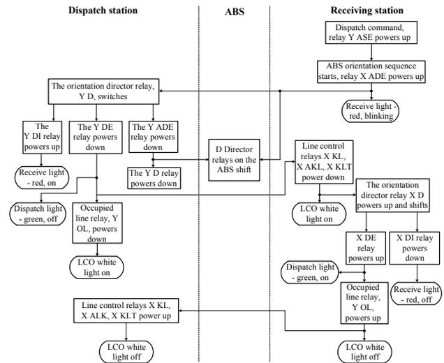
Fig. 2. Operating diagram for the regular inversion of the ABS orientation.
