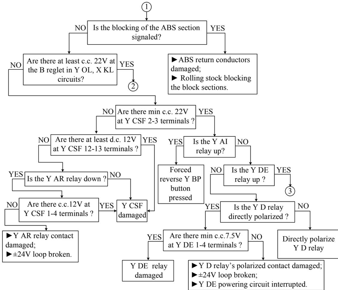
Fig. 3. Failure diagnosis chart for OCL signals in both stations.
