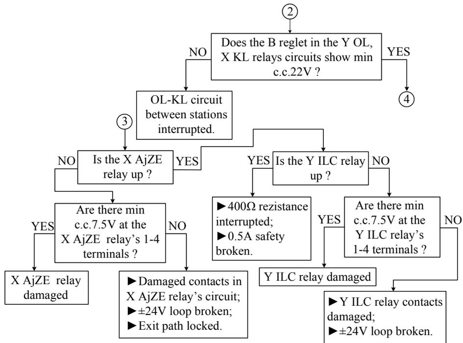
Fig. 4. Failure diagnosis chart for OCL signals in both stations – continued.
