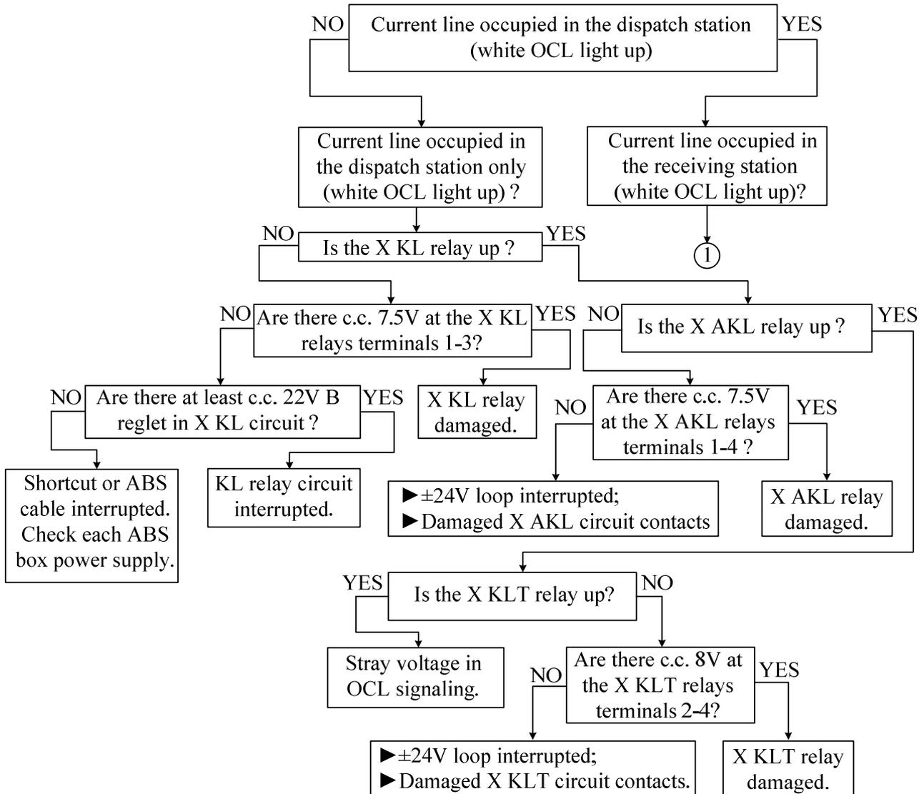
Fig. 2. Failure diagnosis chart for OCL signals in the receiving station only.
