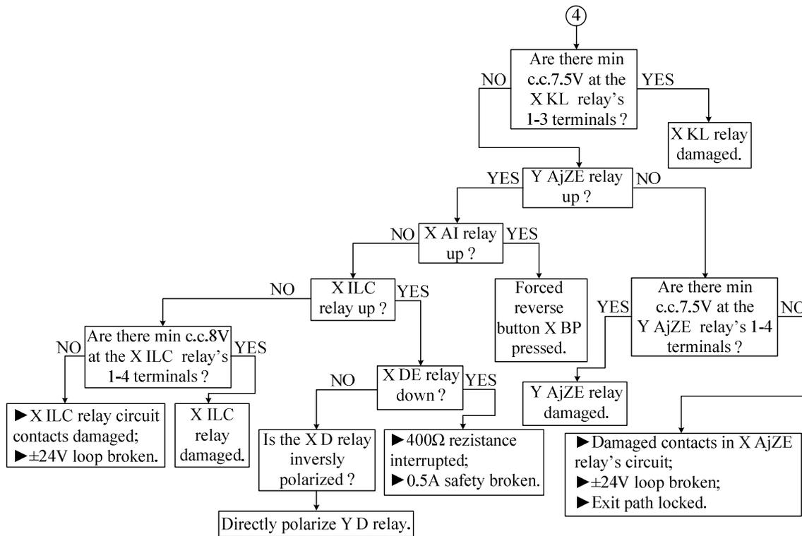
Fig. 5. Failure diagnosis chart for OCL signals in both stations – continued
