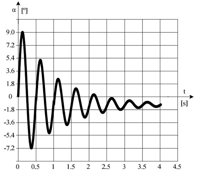
Fig. 3. Time variation of the rotor position angle  $\alpha$  using the functions in relations (25), (26), and (27).
