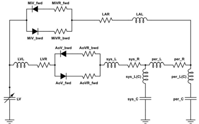
Fig. 1. Lumped parameter model of the mock circulation.
