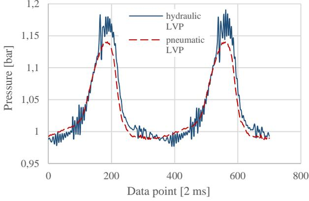
Fig. 4. LVP response with hydraulic and pneumatic actuation.
