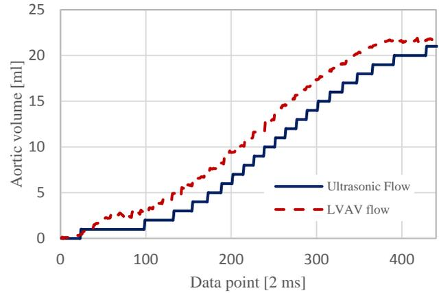
Fig. 6. Comparison of unfiltered measurements using the ultrasonic and newly developed LVAV flow sensing principle.
