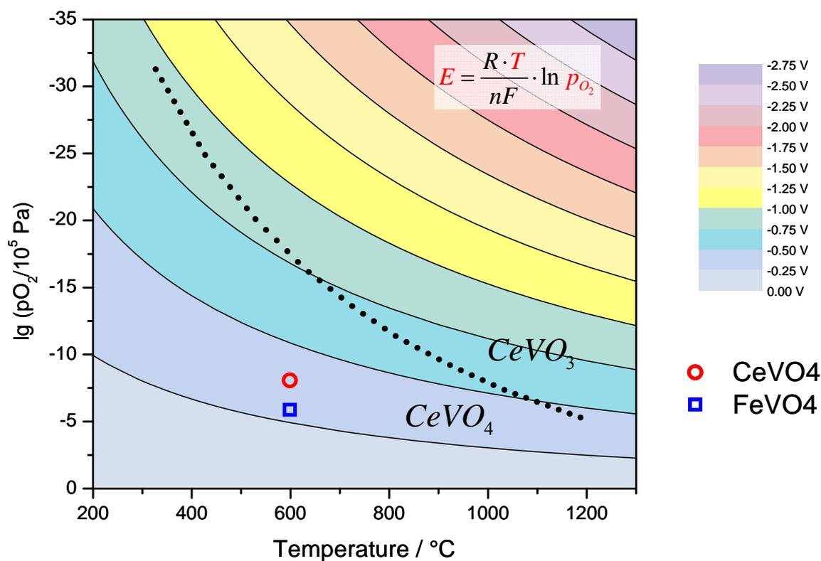
Figure 7. Comparison of measured redox potential (symbols) with calculated stability of  $CeVO_4$  against reduction (dotted line). Contour plot shows the relationship between  $\lg(pO_2)$  and potential of a reversible oxygen electrode vs. the reference value at  $10^5$  Pa as a function of temperature.
