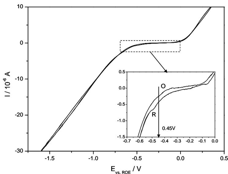
Figure 6. Voltammogram on  $\text{CeVO}_4$  taken at  $600^\circ\text{C}$ .
