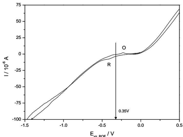
Figure 5. Voltammogram on  $\text{FeVO}_4$  taken at  $600^\circ\text{C}$ .
