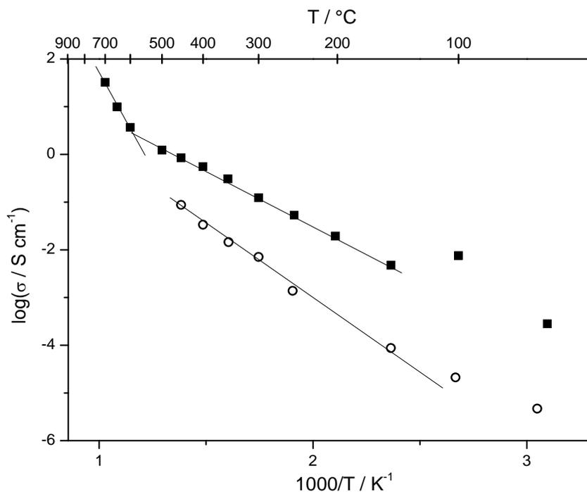
Figure 3. Arrhenius plot of the conductivity for  $\text{FeVO}_4$  (solid rectangles) and  $\text{CeVO}_4$  (open circles).
