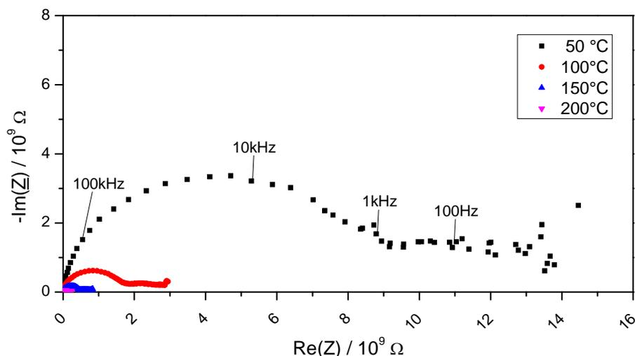
Figure 4. Complex plane plot of the impedance for CeVO<sub>4</sub>.
