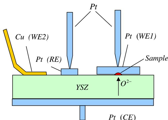
Figure 1. Schematic drawing of the cross-section of the electrochemical cell.
