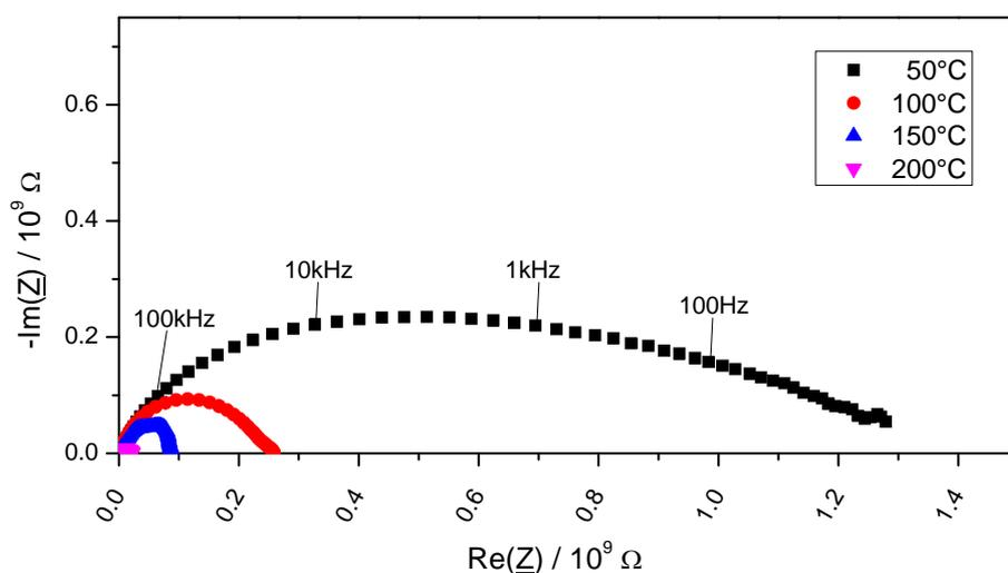
Figure 2. Complex plane plot of the impedance for  $\text{FeVO}_4$ .
