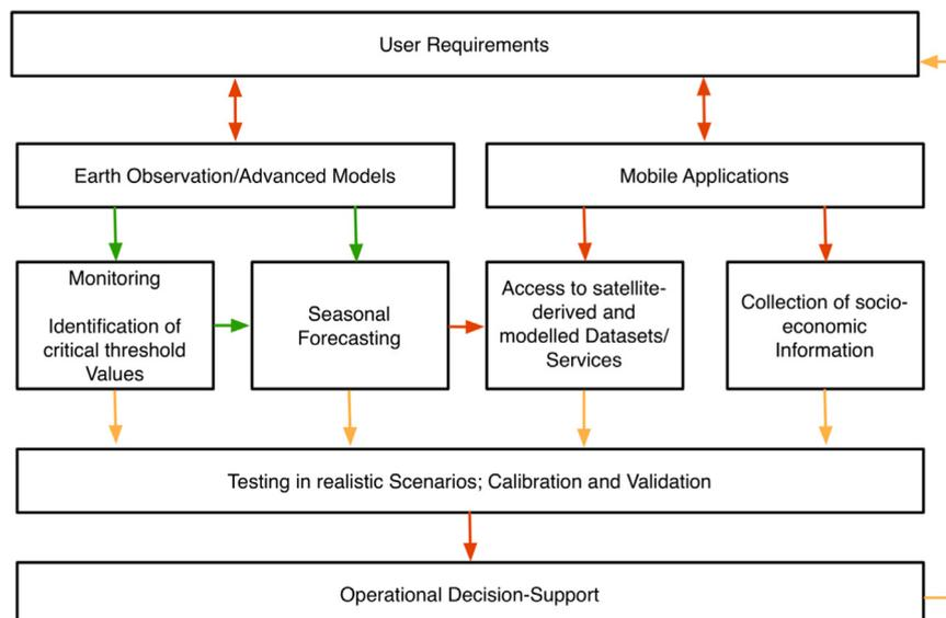
**Fig. 1.** Proposed framework for an operational decision-support system that considers state-of-the-art earth observation, advanced models and mobile applications based on user requirements (established connections are illustrated in green, moderate connections in orange and weak connections in red).
