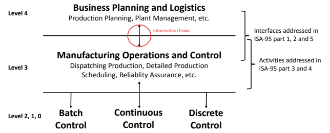
Fig. 1. ISA-95: Functional Hierarchy model [DIN EN 62264-1]
