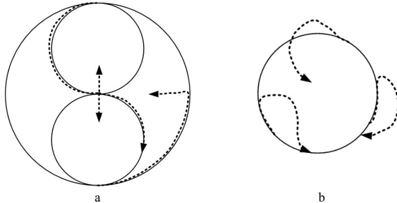
**Fig. 1** Circular redirected walking algorithms. The user is following a circular trajectory with turns that are handled by the algorithms. a – Large circle algorithm. The user stays within the biggest circle. Smooth turns are following smaller circles,  $90^\circ$  turns are supported if directed to the center or started in the center. b – Small circle algorithm. The user walks inside and outside the small circle and is slowly redirected back to the circular trajectory.
