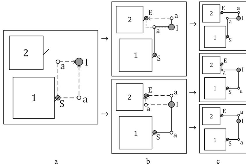
**Fig. 6** The algorithm of flexible spaces. a - An intermediate point *I* is randomly selected and the end point *E* is defined by the nearest door of the target room 2. b - Random selection of point *a* creates a variation of twists of the corridor. c - Several possible corridor routes can be generated from these combinations of points.
