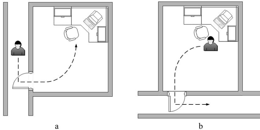
**Fig. 3** Change blindness based redirected walking. a – The user enters a room to perform a task. b – During the task performance the door is relocated in order to keep the user within the tracking space.
