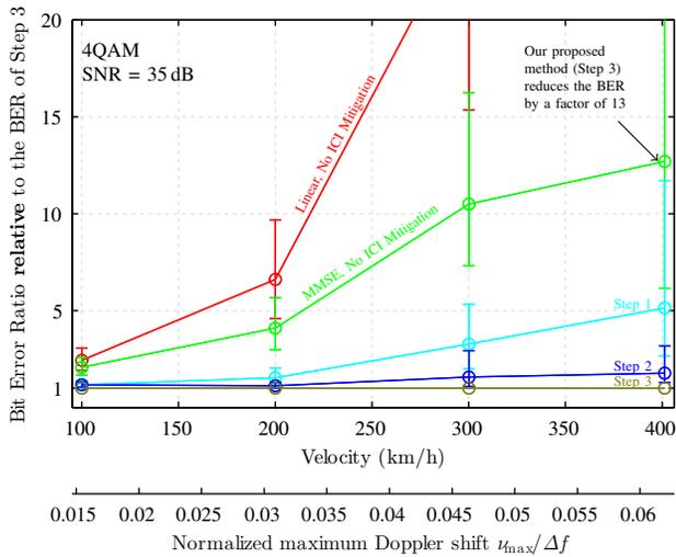
Fig. 5. Measured BER **relative** to the BER of Step 3 as a function of velocity. Compared to Figure 3, the potential improvement of our ICI mitigation method is lower because the underlying channel parameters differ between simulation and measurements (lower delay spread due to indoor measurements, lower Doppler spread and  $N > L$ ).
