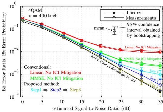
Fig. 4. Measured BER and theoretical BEP as a function of estimated SNR, similar to Figure 2. Also in testbed measurements, our proposed ICI mitigation methods comes close to perfect channel knowledge and no ICI.
