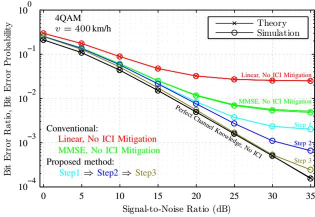
Fig. 2. Simulated BER and theoretical BEP as a function of SNR. Simulation confirms our analytical prediction. At high SNR, our ICI mitigation method avoids an early saturation of the BER. Each step improves the BER and Step 3 achieves a performance close to perfect channel knowledge and no ICI.
