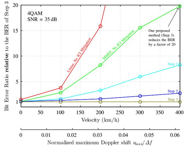
Fig. 3. Simulated BER **relative** to the BER of Step 3 as a function of velocity, respectively normalized maximum Doppler shift. The higher the velocity, the better our methods performs compared to conventional methods. For a velocity of zero, the BER of MMSE (no ICI mitigation), Step 1 and Step 2 coincide.
