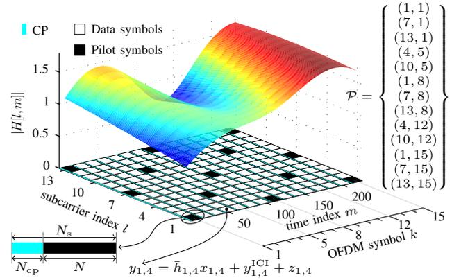
Fig. 1. A possible realization of the sampled time-variant transfer function  $H[l, m]$  for  $L = 13$ ,  $K = 15$ ,  $N = 13$  and  $N_{cp} = 2$ . The data symbols  $x_{l,k}$  are transmitted over a  $L \times K$  frequency-time grid, whereas  $\bar{h}_{l,k}$  denotes the piecewise time average of the channel  $H[l, m]$ . The pilot symbol positions are chosen according to the LTE standard.
