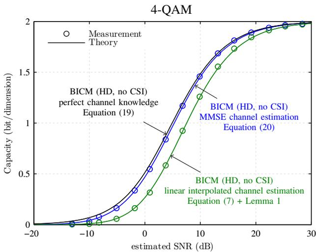
Fig. 4. Measurement results for **4-QAM**. The measured capacities and the theoretical capacities nearly perfectly overlap (within 0.02 bit/dim.), verifying our transmission system model. The performance of MMSE channel estimation comes close to perfect channel knowledge while for linear interpolated channel estimation we find a gap of approximately 2.5 dB.
