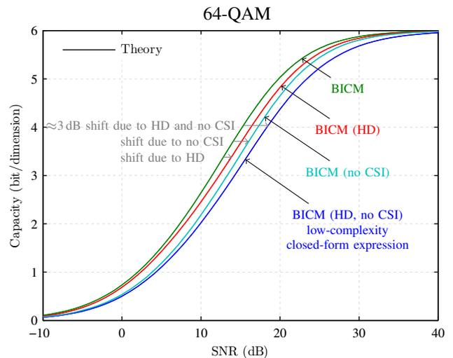
Fig. 3. When comparing our low-complexity closed-form capacity expression with the ordinary BICM capacity for **64-QAM**, we identify a 3 dB shift between these two curves. In contrast to Figure 2, the assumptions of hard decision and no CSI now lead to significantly different capacities.
