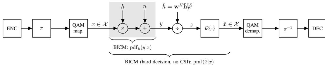
Fig. 1. Block diagram of our BICM transmission system model where  $\pi$  denotes bit-wise interleaving. The ordinary BICM capacity [1] applies the probability density function  $\text{pdf}_h(y|x)$ . We, on the other hand, assume hard decision of the equalized received symbols and that the decoder has no CSI, so that the probability mass function  $\text{pmf}(\hat{x}|x)$  has to be used. Such approach decreases the complexity and allows us to find closed-form capacity expressions.
