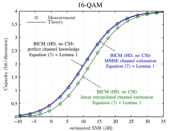
Fig. 5. Measurement results for **16-QAM**. The measured capacities and the theoretical capacities nearly perfectly overlap (within 0.03 bit/dim.), verifying our transmission system model. The performance of MMSE channel estimation comes close to perfect channel knowledge while for linear interpolated channel estimation we see a gap of approximately 2 dB.
