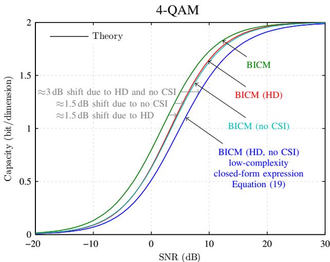
Fig. 2. When comparing our low-complexity closed-form capacity expression with the ordinary BICM capacity for **4-QAM**, we observe a 3 dB shift. Additionally we show how each of our main assumptions (hard decision and no CSI) affects the ordinary capacity.
