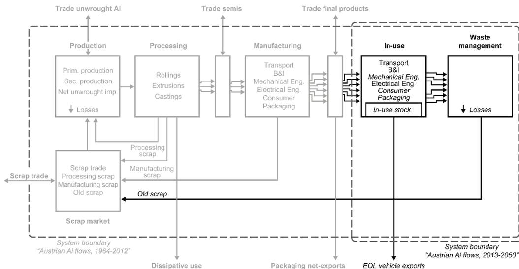
**Figure 2 National dynamic material flow model. System definition after Buchner et al. (2015a)**
