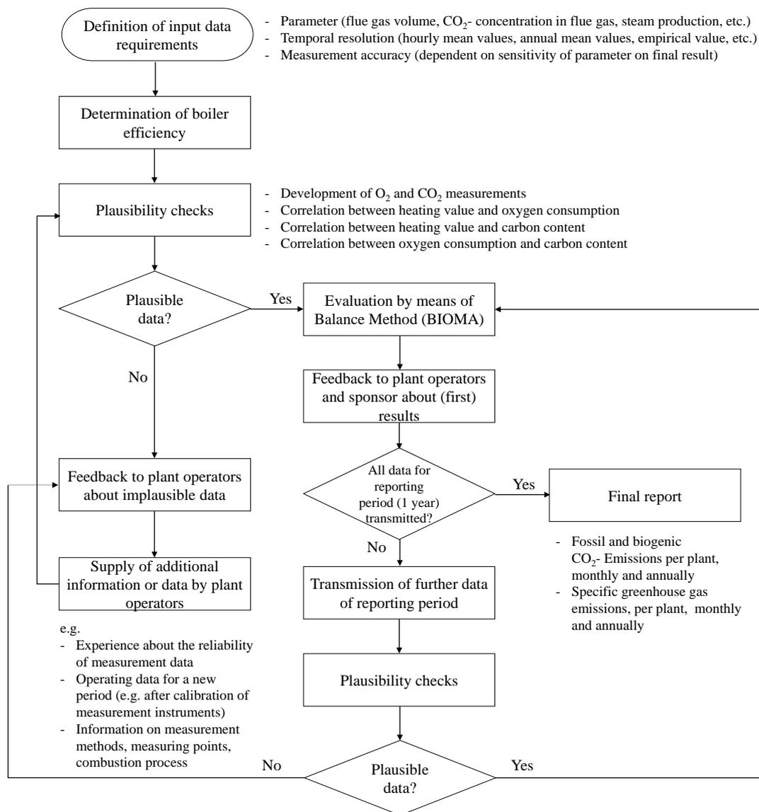
Figure 4. Procedure for the analysis of the operating data of the WTE plants using the Balance Method (software BIOMA) - based on Schwarzböck et al. (2015).
