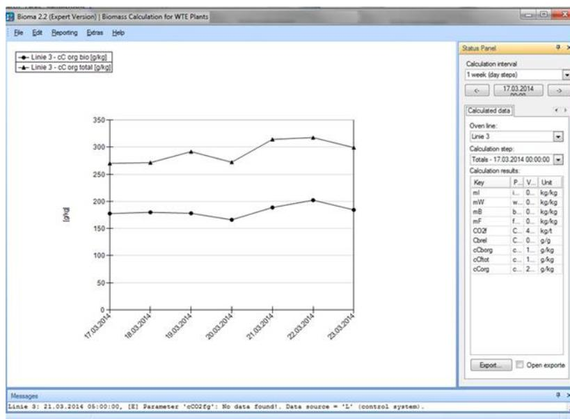
Figure 3. User interface of the software BIOMA (showing daily averages for the total and the biogenic carbon content of the waste feed for a period of one week).
