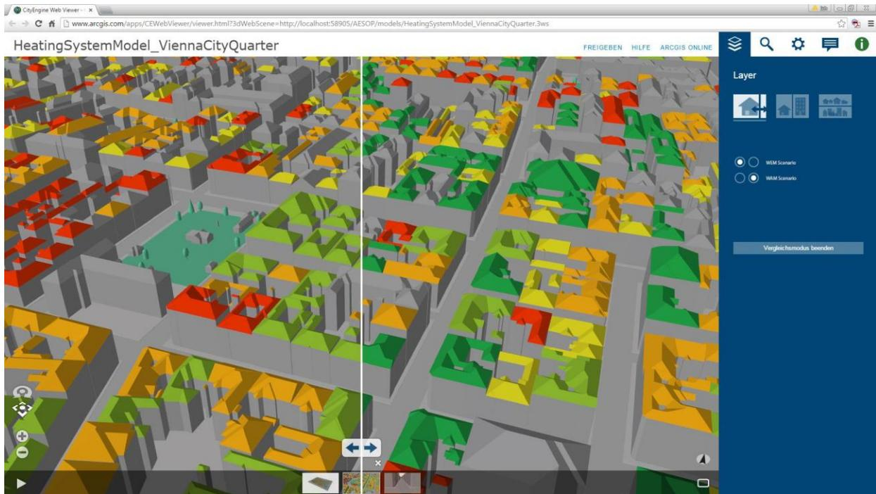
**Figure 5: 3D Spatial simulation with the share of installed solar heat units in comparison to the theoretical potential of installing solar heat units until 2030 for WAM (right) and WEM (left) scenario**
